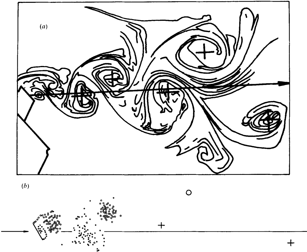
FIGURE 3. (a) Sketch of vortex pattern behind the plate taken from figure 5 of Sarpkaya (1975). Approximate locations of vortices and the free-stream direction are indicated by the plus sign and an arrow respectively; \alpha = 50^\circ , t = 37.0(2a/U_\infty) . (b) Vortex arrangements calculated by MFP; \alpha = 60^\circ , t = 30.6(2a/U_\infty) .
